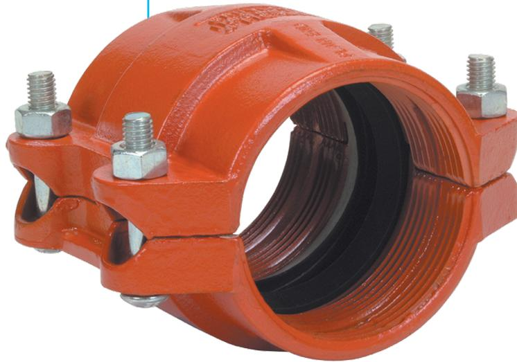
The Gruvlok Figure 7305 HDPE Coupling is a cost effective, easy to assemble, mechanical joint for HDPE pipe conforming to ASTM F714, D2447, D3000, or D3035 with wall thicknesses ranging from SDR 32.5 to SDR 7.3. The Gruvlok coupling method also eliminates the need for costly fusion equipment.
